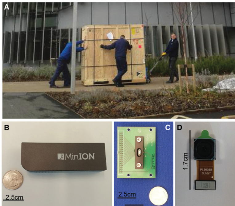
Figure 1. Sizes of sequencing platforms vs. sequencing sensors. For other differences, see Table 1. (A) Three men haul an 860-kg Pacific Biosciences RSII, a sequencing platform, to the University of Exeter (photo courtesy of @PsyEpigenetics). (B) MinION sequencing sensor. (C) An early prototype of a Genapsys flowcell. The company develops an iPad-size sequencer. (D) A commodity digital camera chip ready for cell phone integration. Can DNA sequencers be that small?
