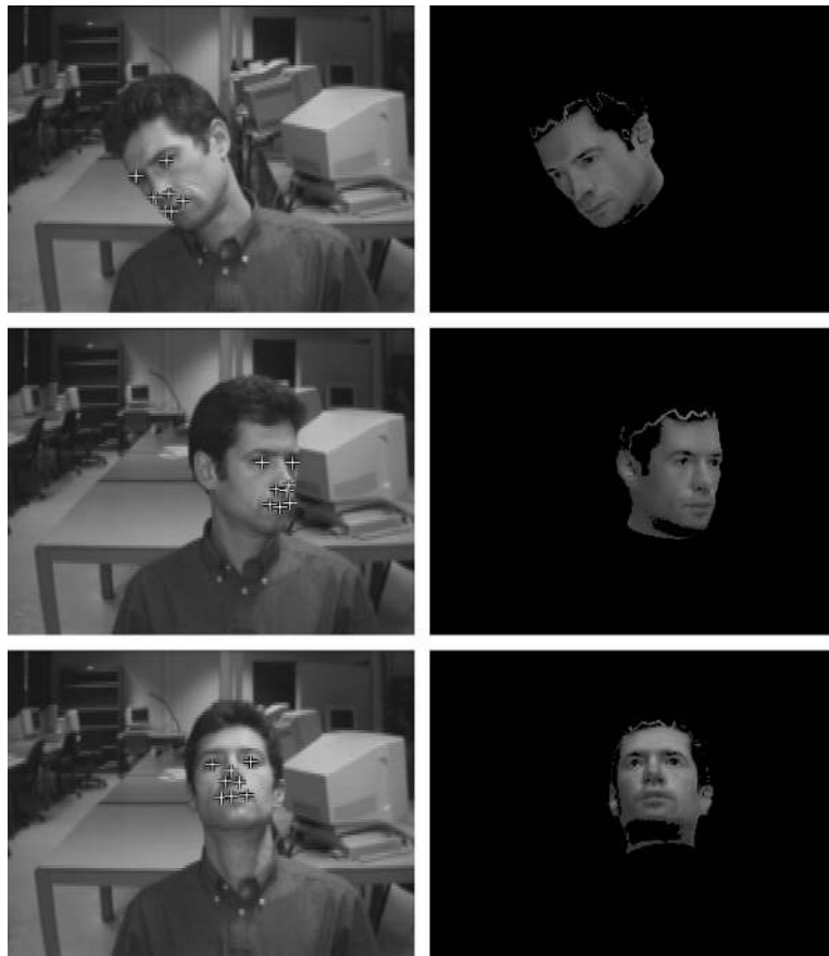
Fig. 11. Head rotations supported by our face tracking system, needing neither markers nor uniform lighting.
