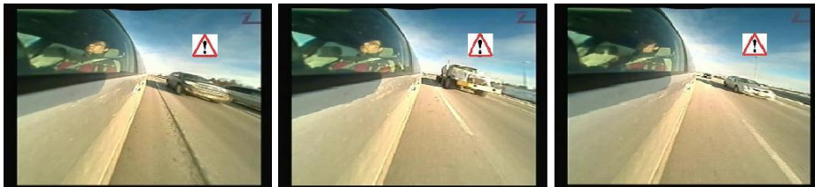
Fig. 5. Blindspot monitoring: The algorithm is efficient in detecting cars of different types and sizes (SUV, truck, standard etc.).
