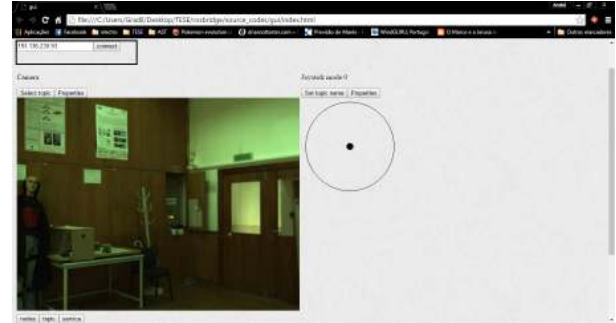
Fig. 10: CASIR-IMPEP remote lab, the HTML web page already connected to the server and streaming one topic.
