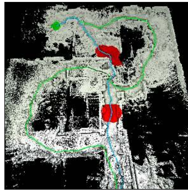
(b) Viable paths through buildings of Tohoku University with two hazardous areas.
