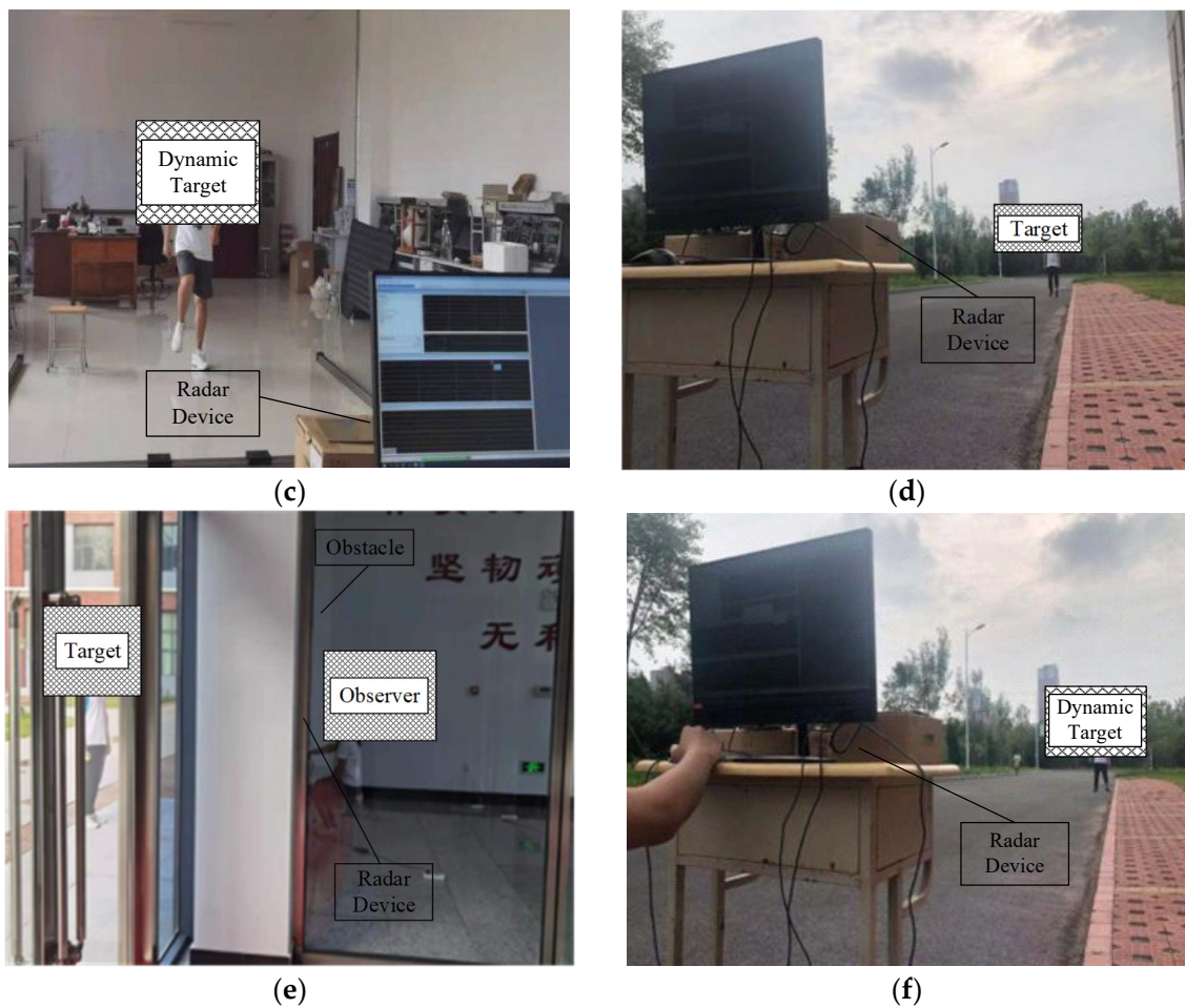
Figure 3. Experimental setup of the system for different scenes: (a) Detection of indoor stationary target; (b) Detection of indoor stationary target covered by obstacle; (c) Detection of indoor dynamic target; (d) Detection of outdoor stationary target; (e) Detection of outdoor stationary target covered by obstacle; (f) Detection of outdoor dynamic target.
