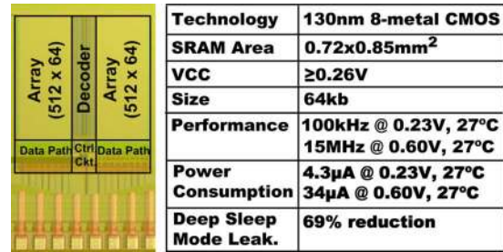
Fig. 23. Chip microphotograph and performance summary.
