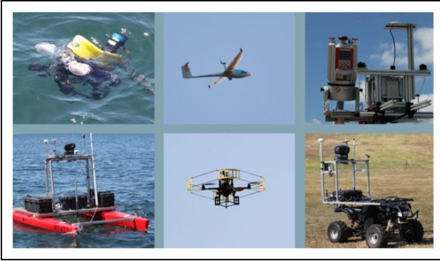
Figure 1. INESC-TEC mobile robotics platforms on land, sea and air application scenarios. All robotic platforms are equipped with one or more visual sensors to perform visual navigation or other complementary tasks.
