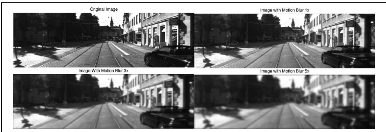
Figure 13. Original image from KITTI data set drive 2011-09-26-0091, and corrupted versions with blur 1, 3, 5 pixels standard deviation denoted as 1\times , 2\times , 5\times .
