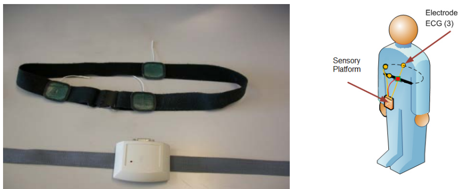
Figure 7. Illustration of R-TIPS. This platform allows monitoring of the cardiac signal wirelessly. It is composed by transmitter system and three sensors (see a).The transmitter system are placed in the participant's hip and the sensors are placed, one in the below right breast, other in the right side and the last in the back (see b).
