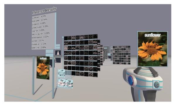
Fig. 2 Representation of CovidResNet in 3D space. Each 2D panel shows the feature maps (channels) of a specific layer. Negative activations are colored blue, zero activations black and positive activations white
