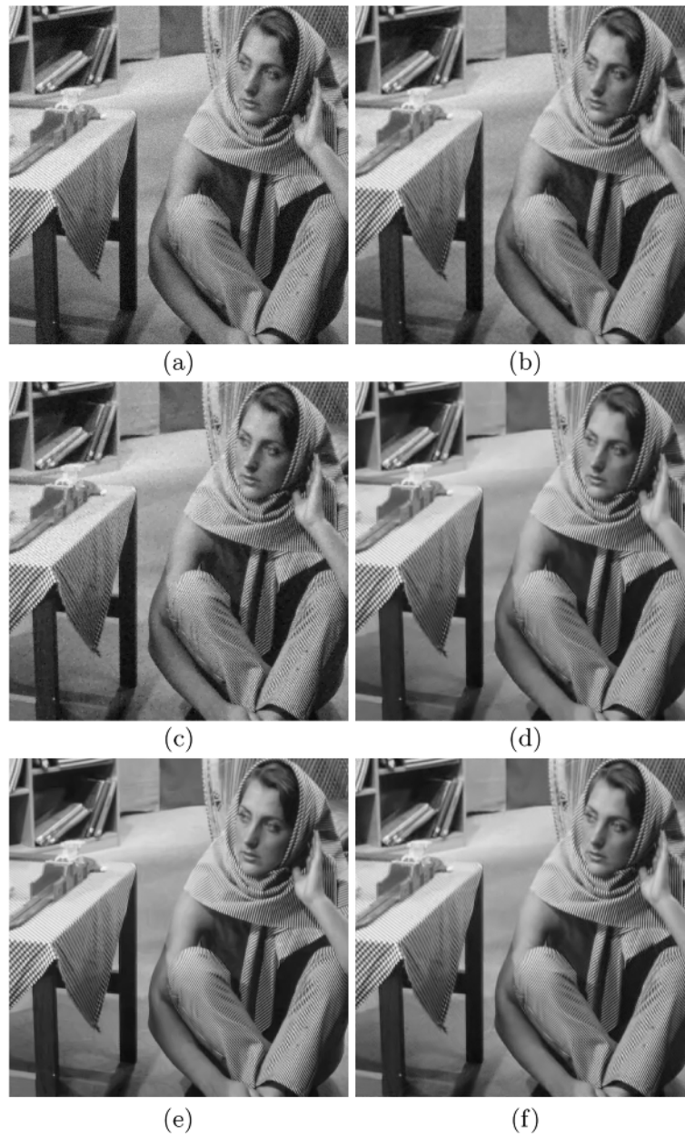
Fig. 5 Denoising performance comparisons of "Barbara" with the noise deviation \sigma = 10 by different methods. a Noisy image. b Denoised image by wavelet thresholding. c Denoised image by TV. d Denoised image by K-SVD. e Denoised image by BM3D. f Denoised image by the proposed method
