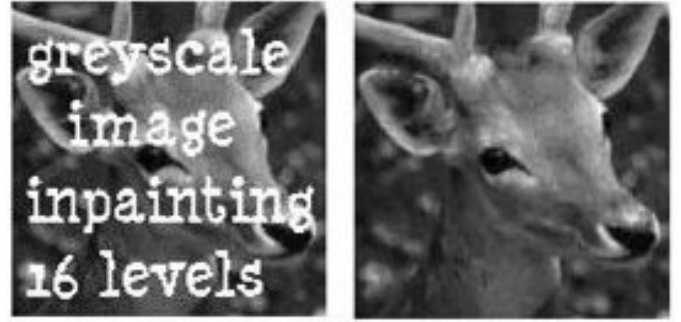
Fig. 6. Grayscale inpainting under occluding text. 5-bit image(16 gray levels) is inpainted after 58 iterations (using Haar wavelet).
