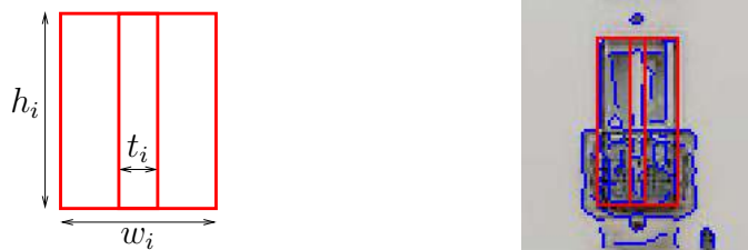
Fig. 2. Left: Window shape template is parametrized by its width w_i \in (0, 1) , height h_i \in (0, 1) , both relative to image height I_h , and the width of the central column t_i \in (0, 1) relative to the window width. Right: Shape template (red) is matched with image edges (blue).
