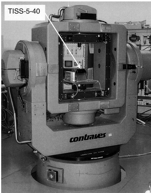
Figure 10. The three-axes rate table that was employed to evaluate for the accuracy of the attitude.
