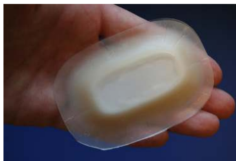
Fig. 1. The “Electronic Patch”. The patch has as a size of 88 mm by 60 mm and is 5 mm thick.
