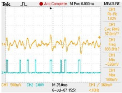
Fig. 6. The yellow (top) graph shows a recorded EMG signal by the Electronic Patch. The blue (bottom) curve indicates the turn on and off of the microprocessor which is controlled by an analog frontend spike detecting circuit.
