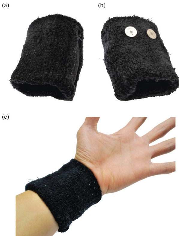
Fig. 3. Wearable EDA sensor. (a) Final packaging in an attractive and inconspicuous wristband. (b) Disposable Ag/AgCl electrodes attached to the underside of the wristband. (c) Wearable EDA sensor can be worn comfortably on the wrist for long periods of time and during daily activities.
