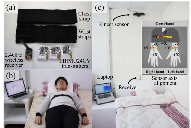
FIGURE 4. System setup: (a) Sensor set (b) A participant wearing sensor sets (c) Sleep experimental room.
