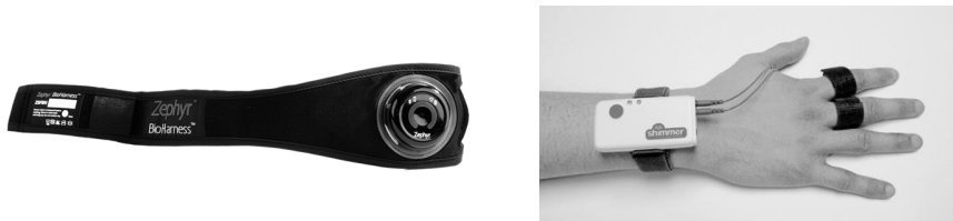
Figure 1. Zephyr BioHarness™3 on the left and Shimmer GSR Sensor on the right
