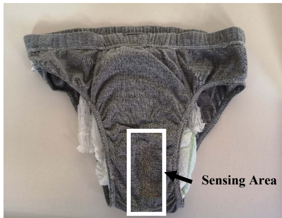
Fig. 2. Embroidered sensor in an underwear with a diaper
