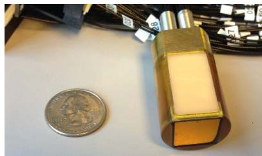
Figure 5-4: Custom two-dimensional transducer array for TCD instrumentation.
