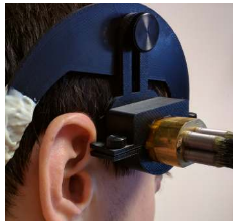
Figure 5-9: Headframe with transducer array translation stage.
