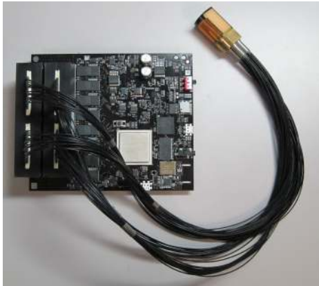
(a) Electrical hardware and custom transducer array.
