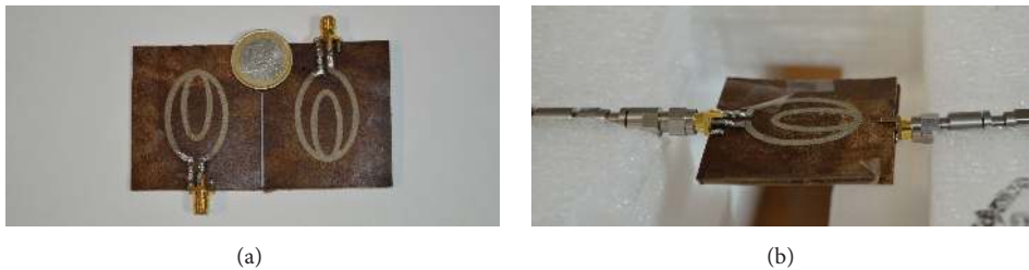
FIGURE 6: Picture of the fabricated prototype: (a) the two resonators; (b) measurements setup.
