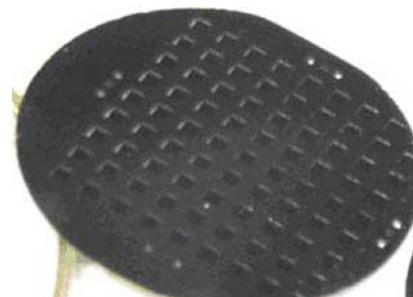
Figure 2 Cavity arrays on one side of the silicon wafer realized in 45 percent KOH at 80^\circ\text{C} till holes are emerged on the wafer edges as shown
