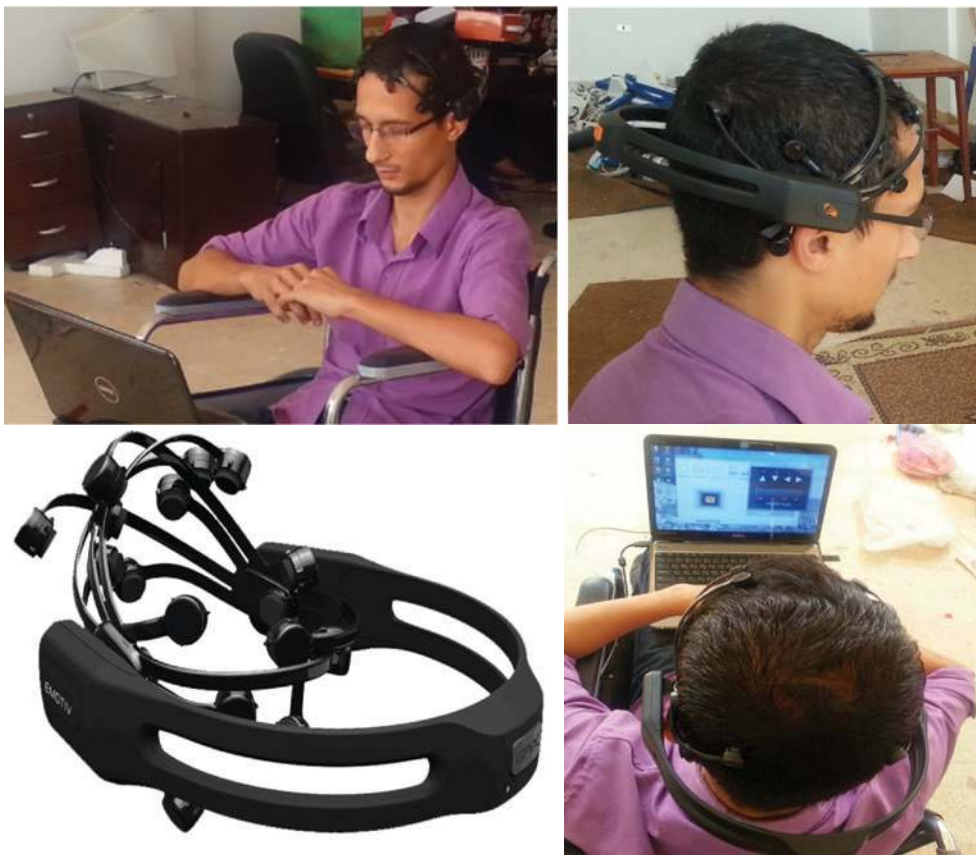
Figure 1: Emotiv EPOC Headset that was used to Control the Intelligent Wheelchair Setup for Assisting the Locked-In Subjects.
