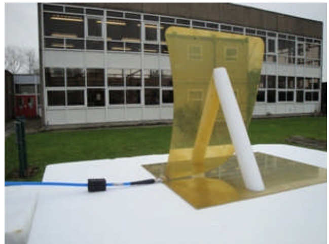
Fig. 8. Free space measurement on an OATS.
