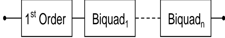
Figure 2.2: Cascade approach to realize a higher-order filter.
