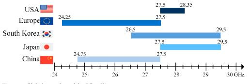
Figure 1. Global snapshot of the 5G millimeter-wave spectrum.
