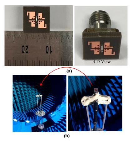
**Figure 4.** Photographs of the proposed CP ME dipole antenna: (**a**) fabricated prototype and (**b**) far field measurement setup.
