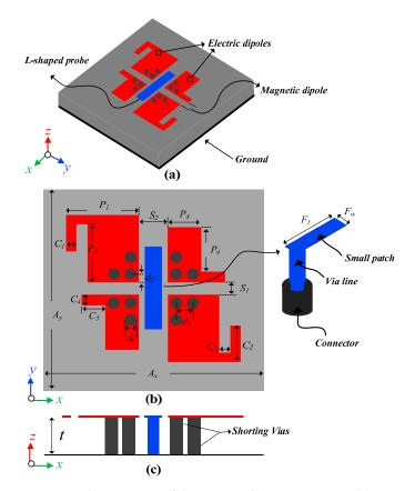
Figure 2. The geometry of the proposed CP ME antenna: (a) 3D view, (b) top view, and (c) side view.
