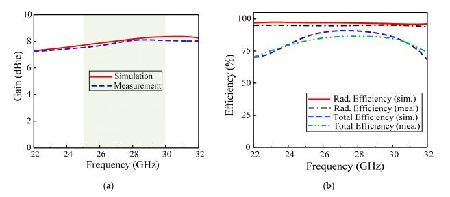
**Figure 6.** Proposed CP ME dipole antennas: (**a**) broadside gain, (**b**) radiation efficiency and total efficiency.
