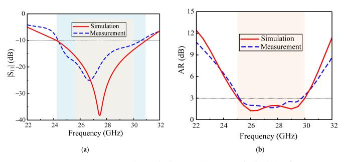
**Figure 5.** Proposed CP ME dipole antenna: (a) S-parameter  $|S_{11}|$  and (b) axial ratio.
