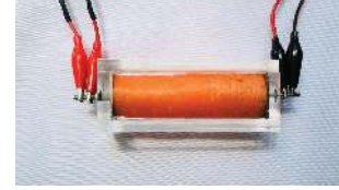
Fig. 19: The carrot cylinder was tested to evaluate the performance using SAS.
