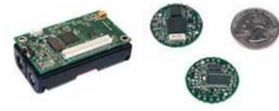
Fig. 3: Crossbow MICA2 (left) and MICA2DOT (right)
