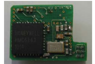
Fig. 4. Micro-IMU bottom view
