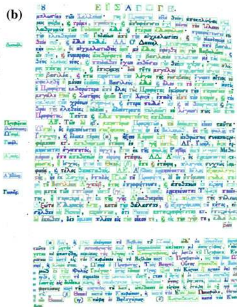
Fig. 3 Applying RLSA to the image of Fig. 2: a after smoothing; b word segmentation result
