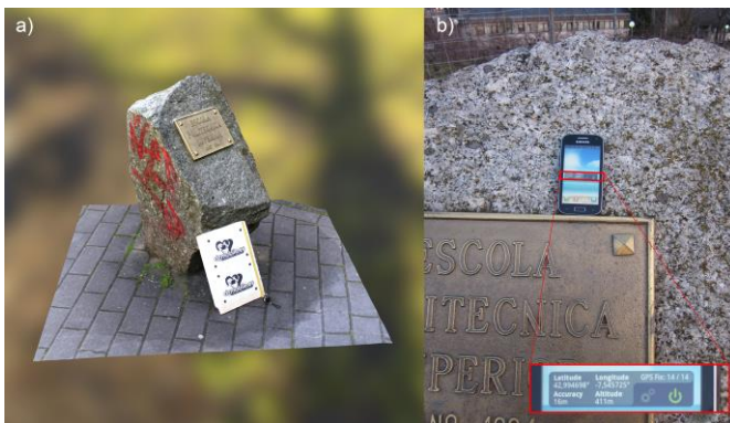
Fig. 2. Free object 3D scanning: fundamentals of photogrammetric 3D reconstruction with images obtained from different angles (a); and GPS data acquisition for model georeferencing (b).
