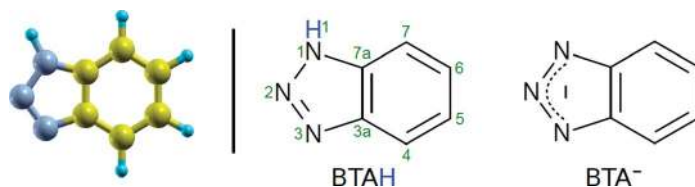
Scheme 1 Skeleton structures of neutral BTAH (middle) and its deprotonated BTA − form (right). Numbering of atoms is also indicated. Ball-and-stick model of BTAH is shown on the left to indicate the respective atom coloring.
