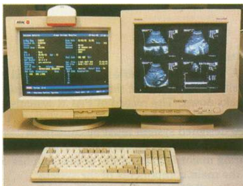
Workstation for a PACS system for ultrasound scans only, with one display screen and a patient data screen.
