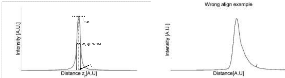
Figure 2. Typical experimental measurement of z vs Intensity (left). Experimental unsymmetrical trace of z_r vs Intensity example due a misalignment condition (right).
