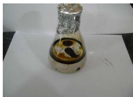
Figure 7. Biodegradation of crude oil by mixed culture of A. niger and A. fumigates after 28 day incubation
