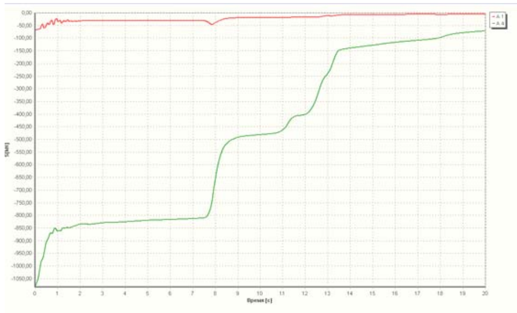
Fig. 10. Value change of the total dynamic additive (upper line) and the total braking force for the entire train, depending on the motion time at regenerative braking movement in prior extended train
