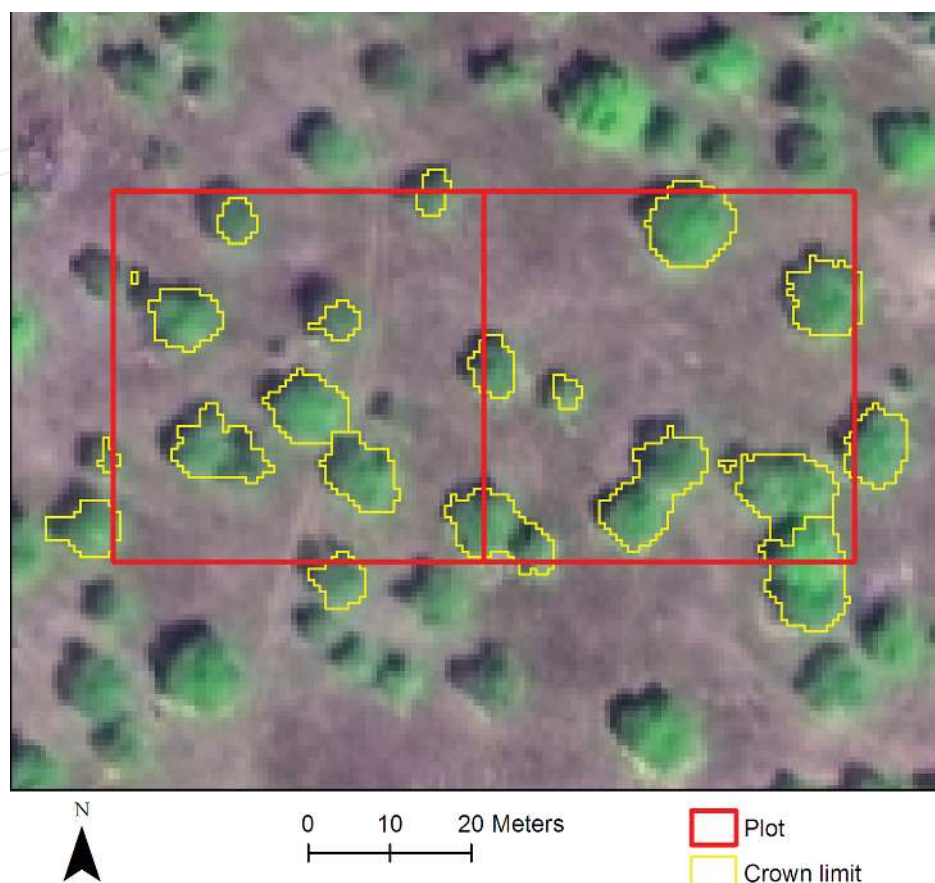
Figure 3. QuickBird image with false colour composite (RGB = red, NIR and blue) and illustration of the results of multi-resolution segmentation process (yellow line).
