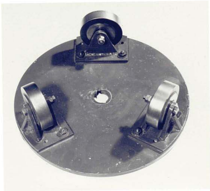
Plate 5.2 The Rolling Wheels Type of Head
