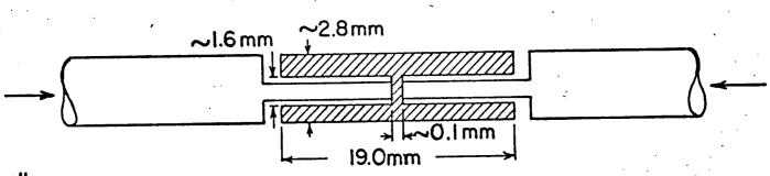
"H" shape core. Core length change correction known and small. Requires spring loading.
