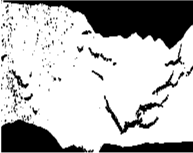
Fig. 8. Quality map relative to the interferogram shown in Fig. 7, part (a), computed using the phase derivative and thresholding procedures presented in [8], Chap. 3. Black color signals pixels where the interferogram is of low quality [8].
