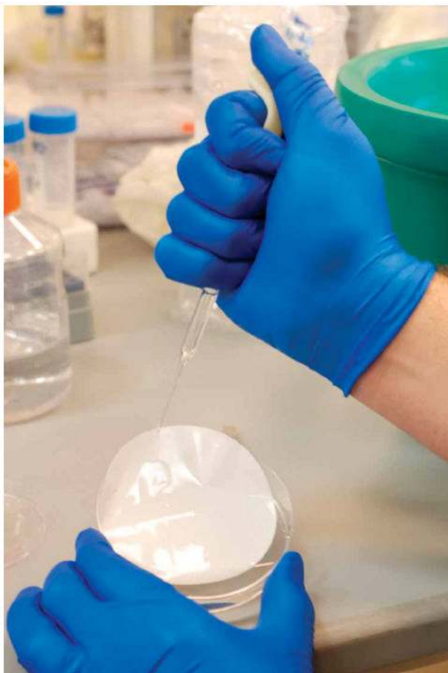
Figure 7. Rinsing the filter with extraction solution (Step 2A(xi)).
