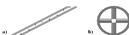
Figure 2. Absorber Tube with Internal Fins ( AFWG_t )
