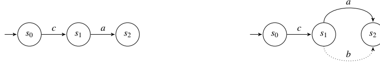
Figure 4.1: The LTS \mathcal{T} (left) is an implementations of the MTS \mathcal{Q} (right).
