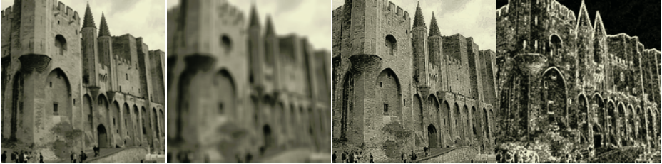
Fig. 1. Examples of image processing convolutions. The original image (left) after blurring, sharpening, and edge detection are performed, respectively ( Image courtesy of Patrick Flynn )
