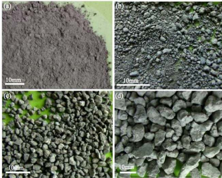
Fig. 2. Optical images of steel slag powders and aggregates: (a) steel slag powders; (b) and (c) <5 mm fine slag aggregates; (d) 5–16 mm coarse slag aggregates.
