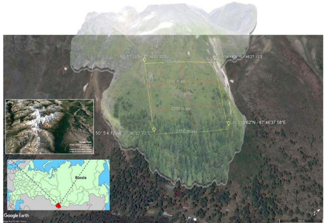
Figure 1. A 3-D model (built by meshing 10 aerial photographs taken by a drone) of the study site on the mountains slope above the Aktru Research Station in the Altai Mountains of Russia (small inset). The model is overlaid on the most recent available (2017) satellite image of the area to show the sampling scheme composed of three vertical and four horizontal transects, placed at a 50-m distance. The geographic coordinates at the corner of the study sites and the altitudes are shown. The smaller inset shows the continuous forest belt between the Severo-Chuyskiy Mountain Chain (white mountaintops on the left) and the Kuray Valley (sandy terrain on the right). The highest altitudinal treeline level is reached at the study site (red arrow) of the Aktru Research Station (inset orientation is the same as the larger satellite image; map data of the inset: Google Earth, Landsat/Copernicus, CNES/Airbus, Digital Globe). The original satellite imagery, obtained from Google Earth Pro® version 7.3.2.5491 ( https://www.google.com/earth/ ; map data: Google, CNES/Airbus), was modified with MeshLab and Sketchup software.
