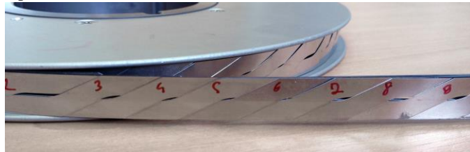
Fig. 2. Roebel cable, 20 m, dummy stainless steel, supplied by Karlsruhe Institute of Technology Institute for Technical Physics (KIT).
