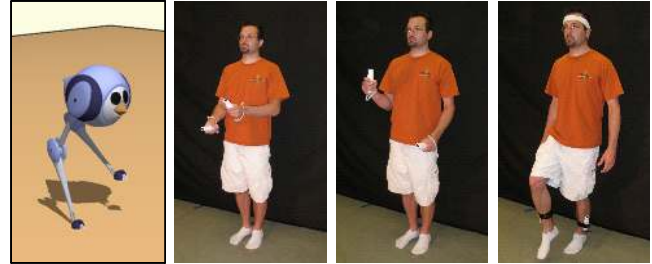
Figure 1: A user controlling a physically simulated bird character with the three Wiimote interfaces: wrists, arms, and legs.
