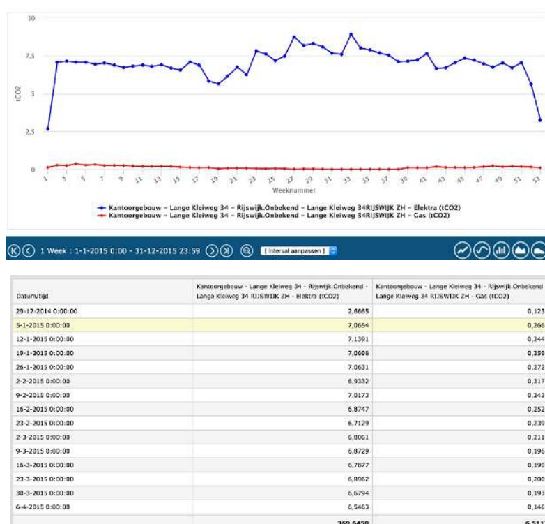
Figure 6: Output-sheet of the eSight tool, regarding the energy consumption in the living lab in 2015
