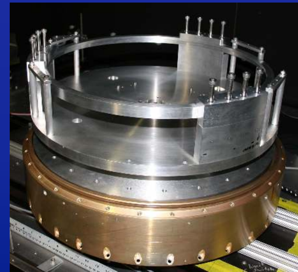
Mirror mount with mating vacuum mount.
