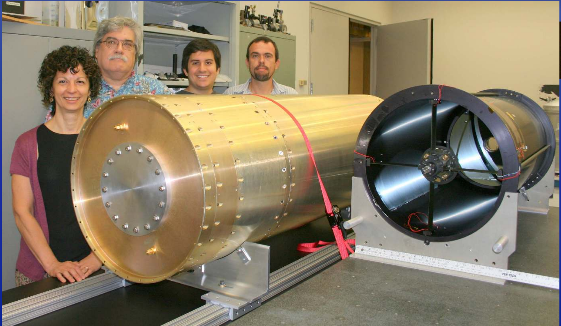
“Artificial star” vacuum housing (left) and collimator component (right).
